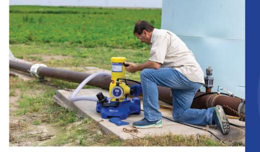
The self-contained design of the MacRoy Series G pump makes it easy for one person to handle and convenient to move from one system to the next.
